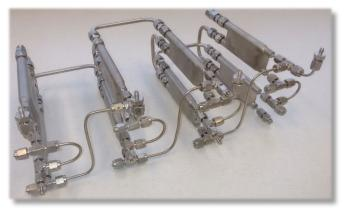
Modular design allows for flexible and fast (re)configuration of the reactor system
